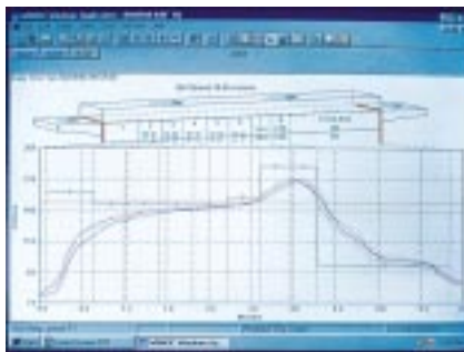
Figure 1. Thermal profiling software records events taking place during the thermal process and displays them for immediate viewing or stores them for later recall and analysis.
