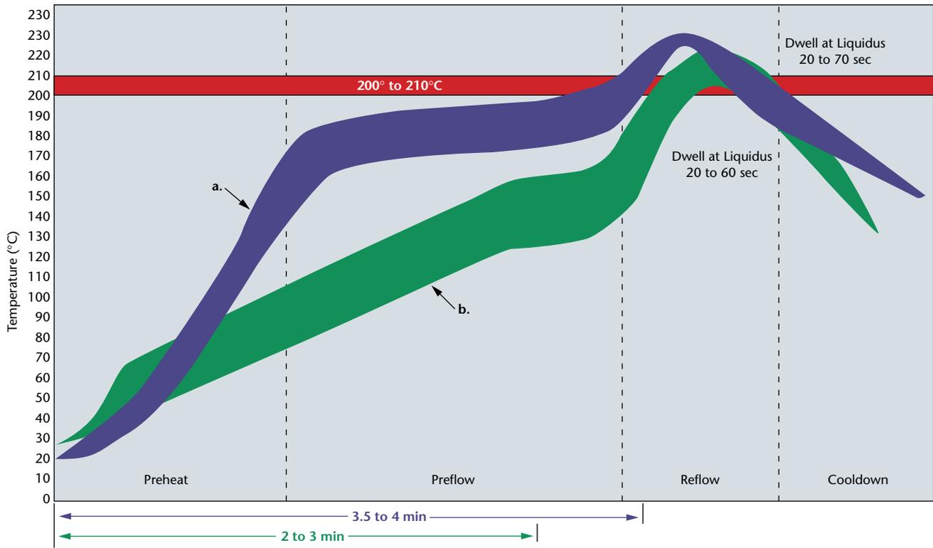
**Figure 1.** The “standard” reflow profile (a) is compared to the “tent” or “straight ramp” pattern. While the former is suitable for solder pastes that require dwells at specific temperatures, the growth in the use of no-clean pastes demands more controlled high temperature periods lest the flux be depleted.
