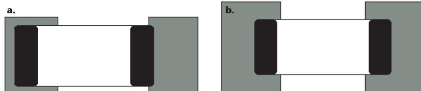
**Figure 2.** Conditions that lend to the possibility of component tombstoning during reflow include inaccurate placement (a) in which a greater wetting force at one end serves to erect the opposite end, and (b) excessive pad size vs. the part’s terminal size, leading to the same effect.
